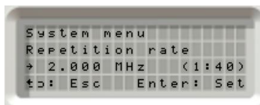
Figure 7-6: Changing Repetition rate
