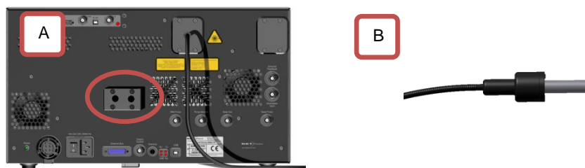
Figure 4-6: Collimator holder (A) and collimator (B)
